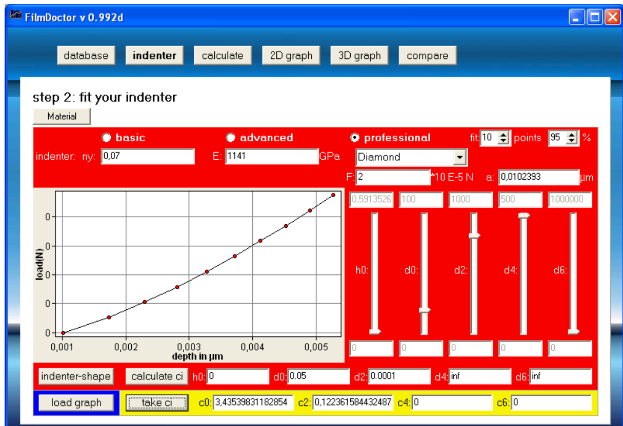
Fig. 2: Load-depth-curve for the ACCU-tip of fig. 1 pressed into a coating-substrate-compound with a maximumload of 20μN.
