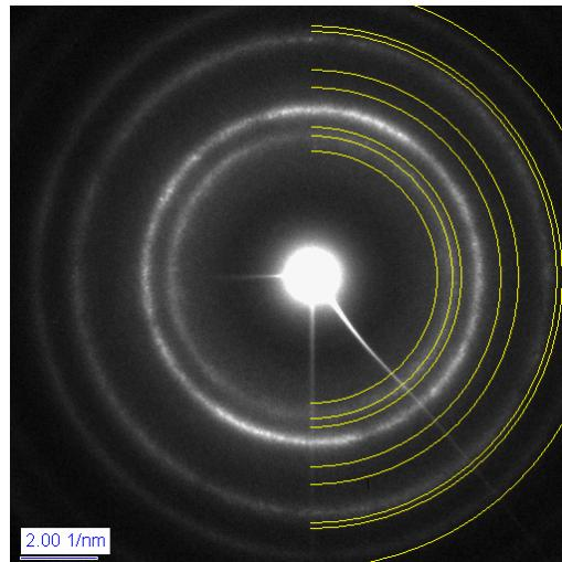
Electron diffraction patterns for standard TaN compared with theoretical patterns (yellow) for the fcc (left) and hexagonal phase (right).
