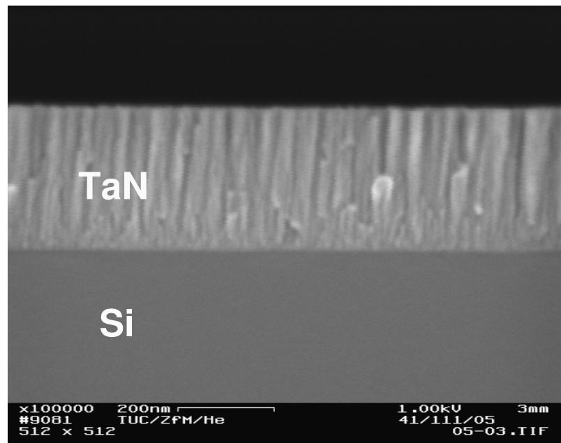
Cross-sectional SEM image of 290nm thick TaN film on Si.
