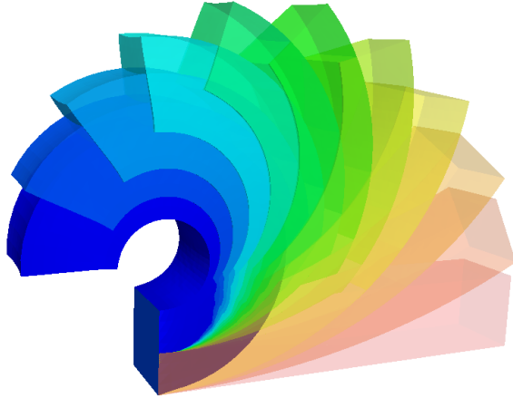
FIGURE 5.4. Solutions of the example 5.4.1 for the load increments s = 0, \frac{1}{10}, \frac{2}{10}, \dots, 1 . The dark blue mesh is the solution for the incremental s = 1.0 while the transparent red mesh in the lower right corner is the undeformed body, i. e. s = 0 .
