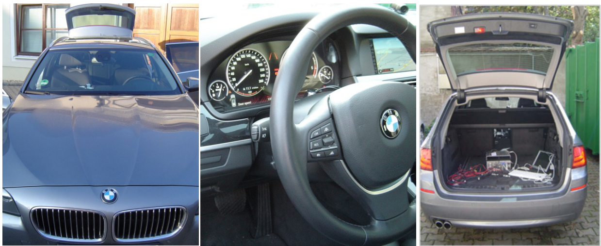
Figure 19. Experiment vehicle with video cameras and data acquisition system.
