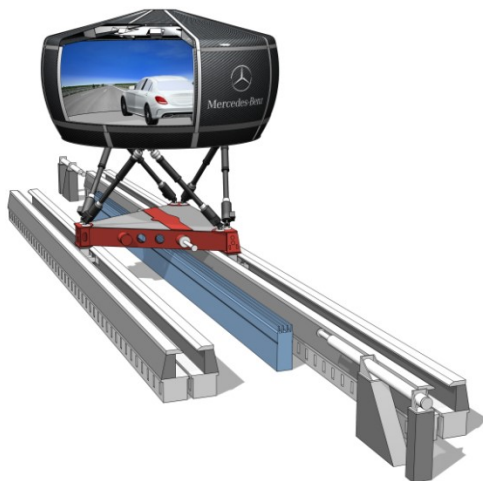
Figure 11. Illustration of the moving-base simulator.
