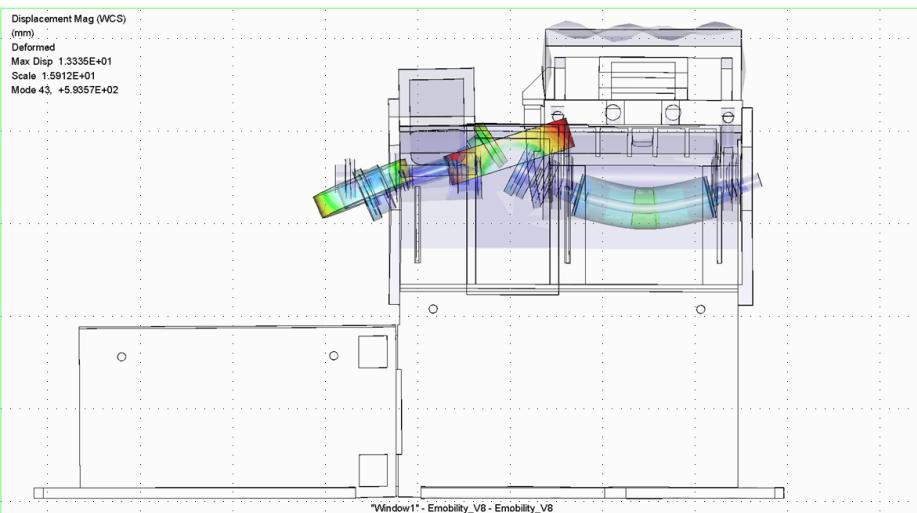
Test bench for **rotary oscillation damper** in the converter gear rotordynamic drive train
