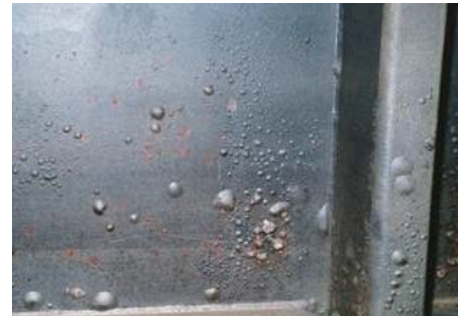
Figure 23. Localized blistering on a coated metal structure. Amtec [161].
