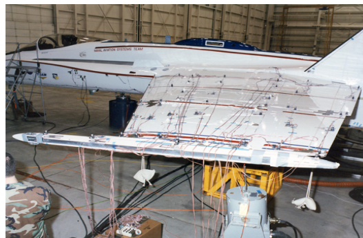
Figure 2.1: Strain sensor array installed on NASA aircraft [2] Credits: NASA / Tom Tschida
