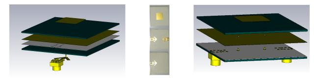
Figure 6.1: Layer set-up of squared microstrip patch antenna design. Left: Single probefeed patch. Center: constructed patches. Right: Differential probe-feed patch
