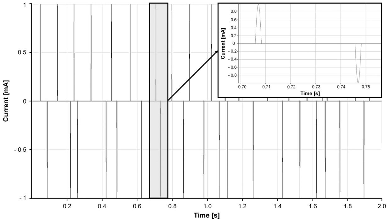
**Fig. 3.** Extract (2 s) from the signal-time curve of the stochastic biphasic current. The normal graphic shows the randomized pause times (10–100 ms) between the pulses. The zoomed graphic shows the short triangular pulses of 1 ms duration.
