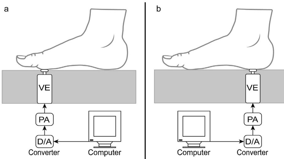
**Fig. 2.** Vibration perception threshold measurement at the first metatarsal head (a) and heel (b). The corresponding anatomical region could be precisely placed over the probe of the vibration exciter (VE). PA: power amplifier; D/A Converter: digital to analogue converter.
