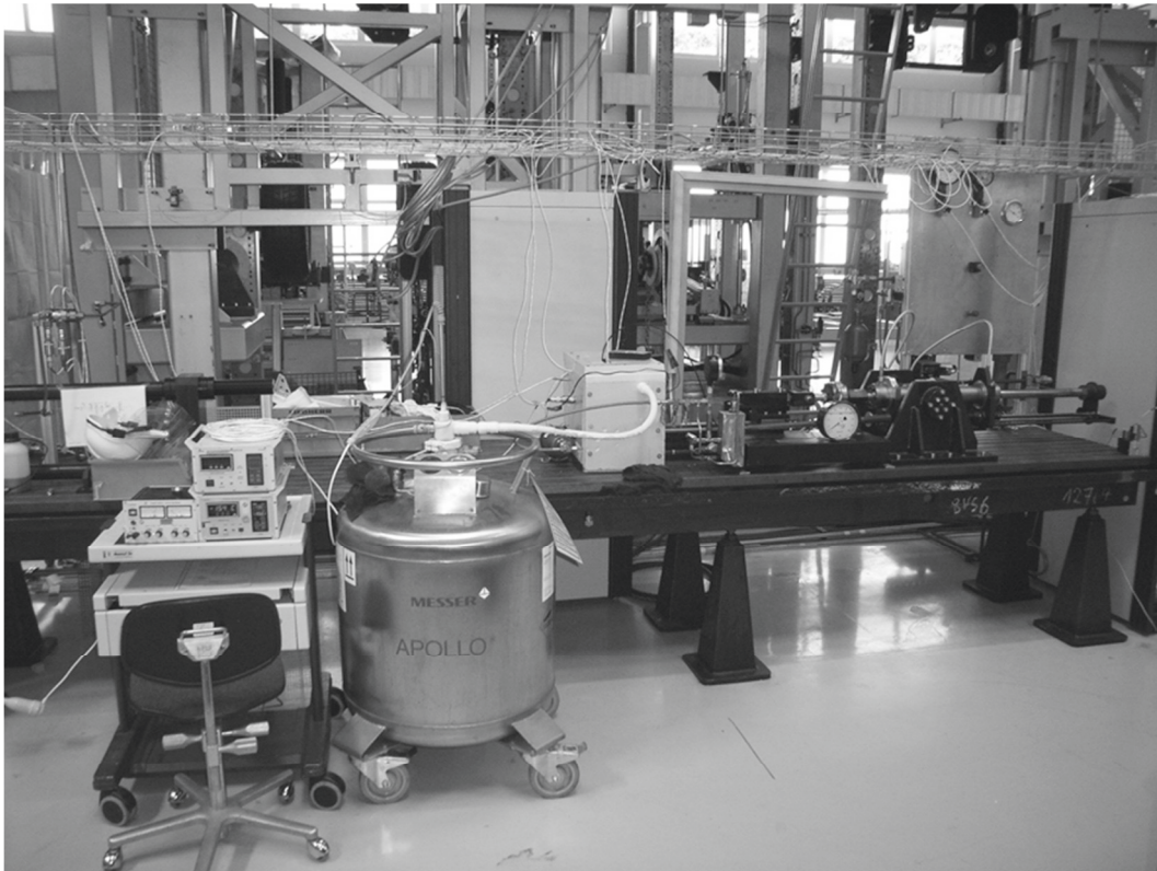
Fig. 7-21: An insulation chamber and cryogen chilling system for low temperature tests
