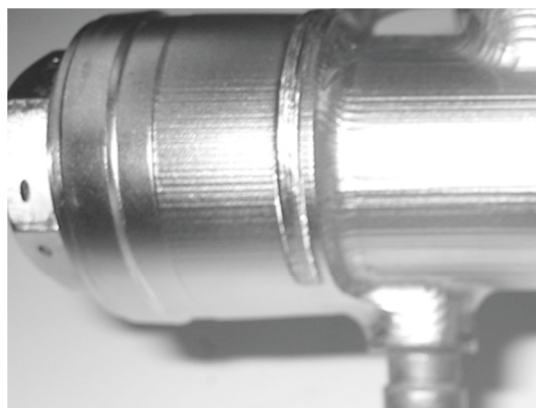
Fig. 7-8: Tear repaired - a Laser welding seam
