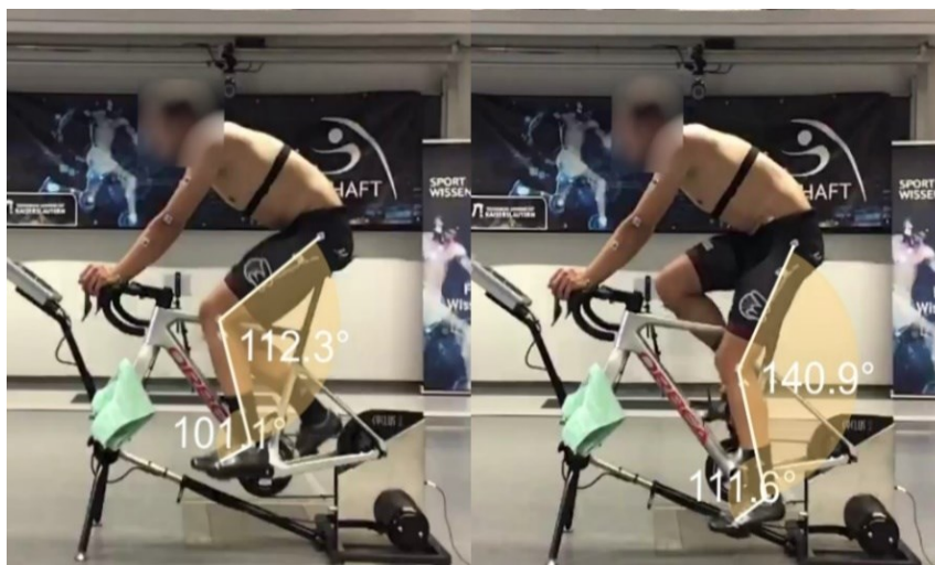
Fig. 1 Measuring procedure and angle definition (metatarsophalangeal joint, the lateral malleolus, the lateral part of the articulation genou and the trochanter mayor)
