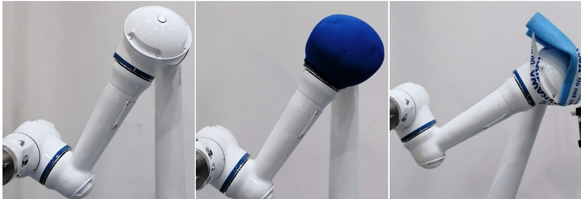
Figure 4.18: Setup for Transient Contact with the Elbow Big Cap – without Padding (left), with Neoprene (middle), and with Foam (right)
