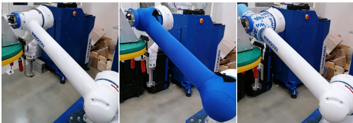
Figure 4.19: Setup for Transient Contact with Elbow Small Cap – without Padding (left), with Neoprene (middle), and with Foam (right)
