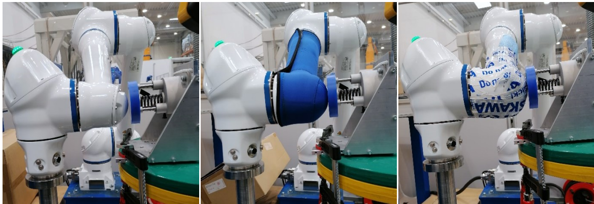
Figure 4.21: Experiment on Transient Contact with Wrist Cap – without Padding (left), with Neoprene (middle), and with Foam (right)
