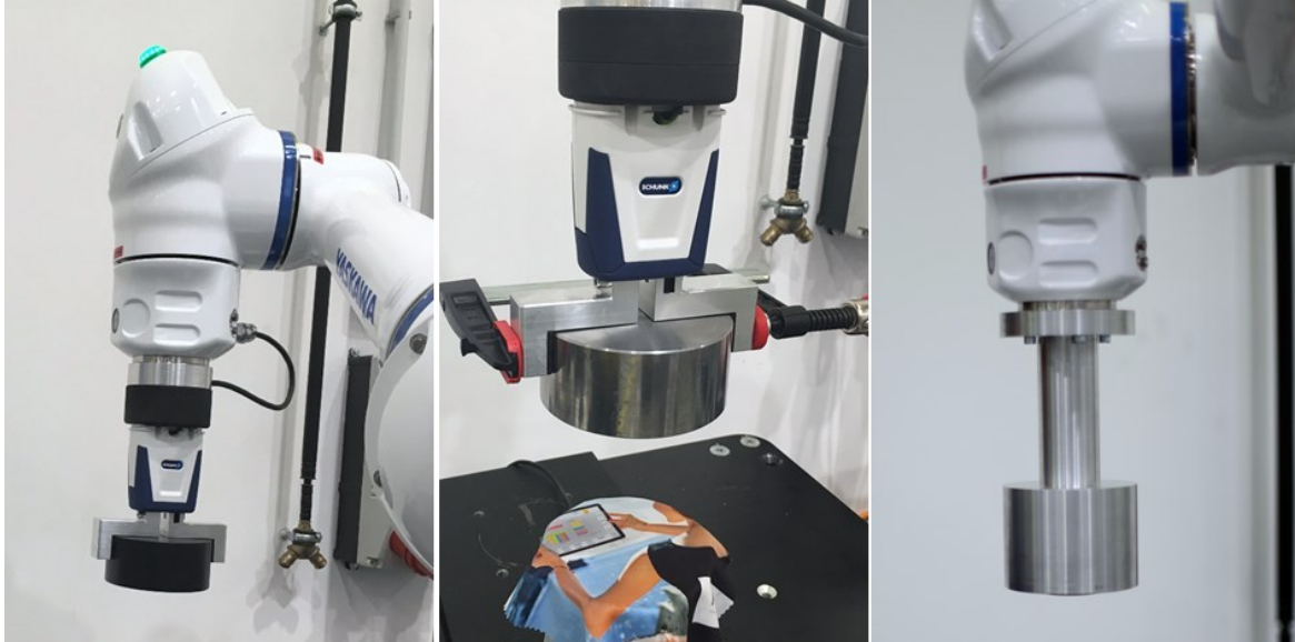
Figure 4.12: Selected Tested Gripper and Workpiece Setups - Schunk Gripper with 50 mm long POM Material (left), Schunk Gripper with 50 mm long Steel Workpiece and Screw Clamp (middle) and Aluminium Basis Workpiece (right)
