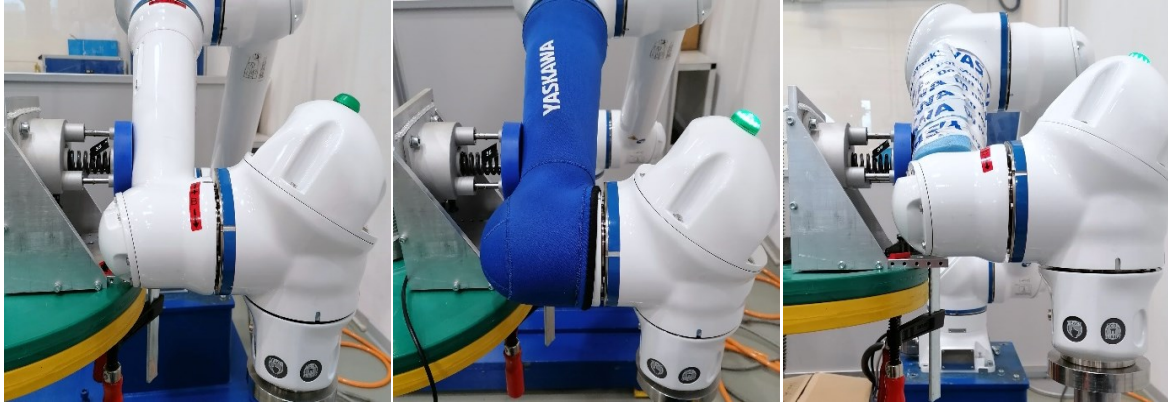
Figure 4.20: Setup for Transient Contact with Forearm – without Padding (left), with Neoprene (middle), and with Foam (right)
